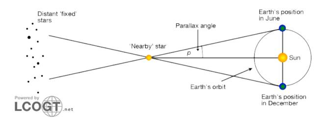
Here in the graph, the distance from the Earth to the Sun is declared to be one astronomical unit(1 AU in calculation). Therefore, we can easily find the relations between the Parallax angle and the distance to star by using the trigonometric rules<sup>5</sup>:
