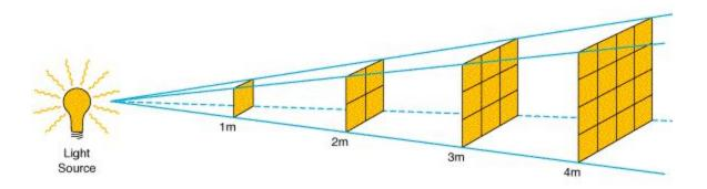
As one can see through the above picture, the luminosity is the energy of light in the light source, while the flux is the energy of light in the yellow panel<sup>7</sup>. Moreover, scientists even found the relations among flux, luminosity and distance, that:
