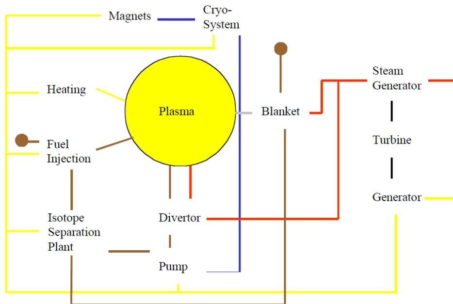
Figure 10: Flow chart for a future fusion reactor: fuel (brown), electrical power (yellow), heat (red), neutron (grey), mechanical power (black) and cooled helium (blue).
