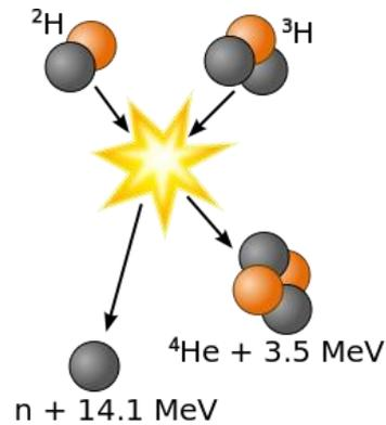
Figure 4: Schematic of the fusion reaction in which deuterium and tritium form a helium atom and a neutron. Mass is lost in the reaction and energy gained.
