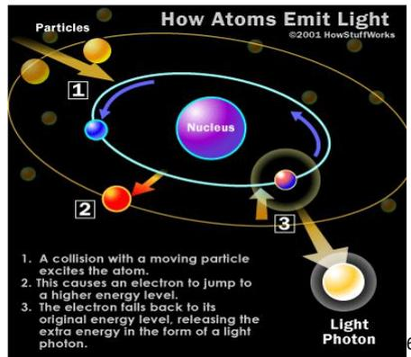
During this procedure, the particles will bombard with gas atoms. These collisions will excite the atoms. Since the atoms gain plenty energy from the collisions, the excited atom is unstable. To transfer these unstable excited atoms into a more stable form atom, the atoms need to release the energy. The carriers of this energy are the photon. Below, we have a function which can measure the energy of the photon.
